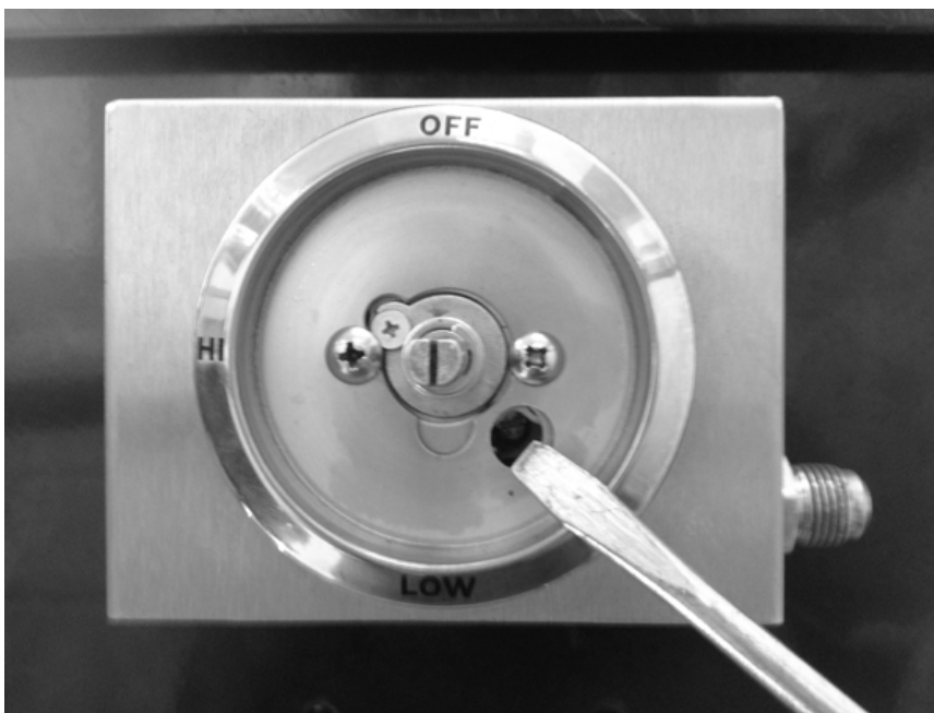
“LOW” Flame setting adjustment screw.
